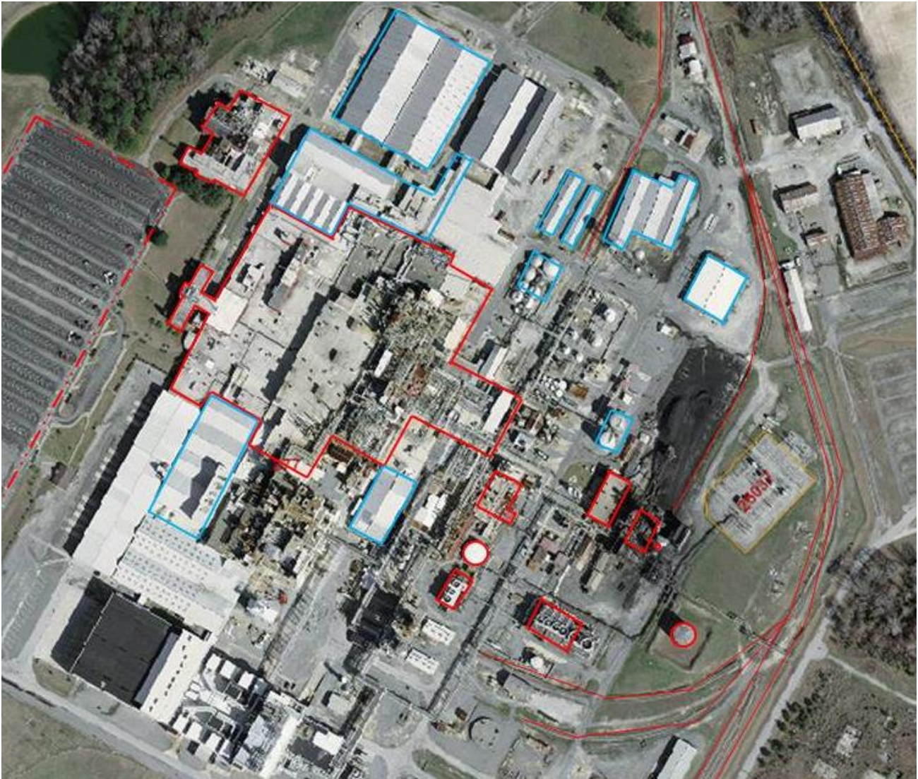
Figure 59. Modern aerial view of facility; buildings outlined in red, including rail lines and parking lot at left, in place by 1954; buildings outlined in blue in place by 1965
